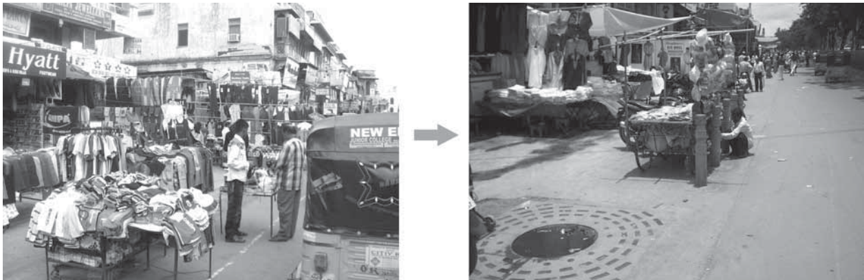
Street vendors on the Madina-Pathergatti Stretch before and after redevelopment in the Charminar Precinct, 2010. The tree pit in the foreground with the tree grate was designed for providing shade to the street vendors and pedestrians. The bollards were designed as segregation for motorised vehicles, five metre carriageway and as furniture for street vendors
