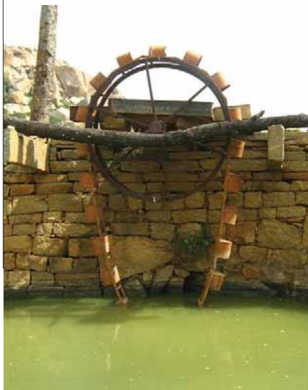
The Persian wheel, locally known as rahat is a water lifting device, with a number of small pots attached to a long chain. The system operates through rotational motion of two gear wheels.
