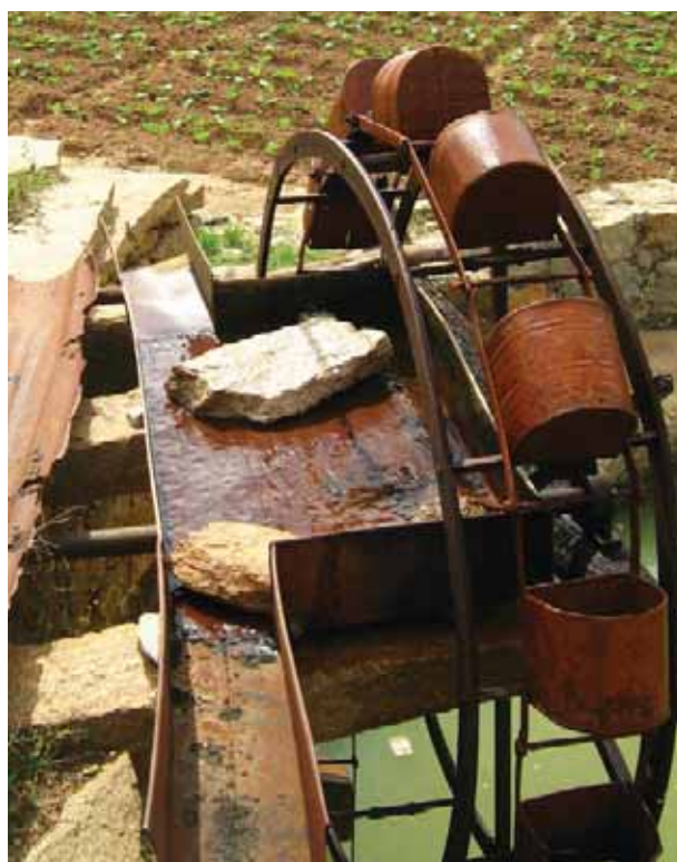
The rahat is used to irrigate agricultural fields, though this practice has all but disappeared, due to the advent of the tube well
