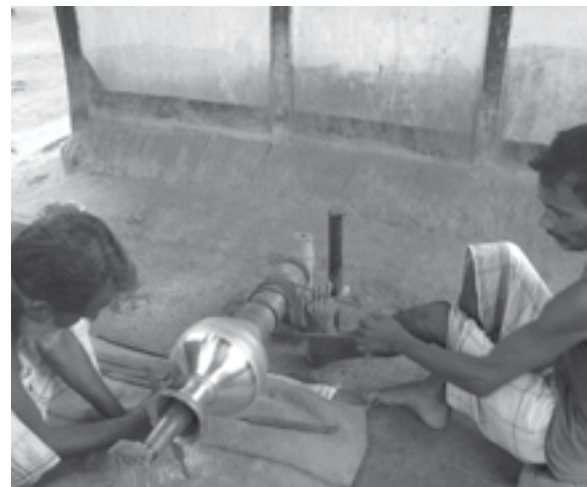
Scraping in progress
