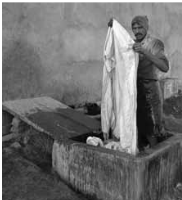
Process of soaking cloth in yellow myrobalan solution
